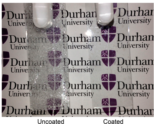
Figure 4. Demonstration of antifogging following exposure to water vapor (fogging): on an uncoated glass slide and a poly(Et- alt -MA)–fluorosurfactant complex solvent cast from DMF. Similar behavior was observed for poly(St- alt -MA)–fluorosurfactant and poly(St- co -MA)–fluorosurfactant complex dip-coated glass slides using a DMF solvent.
